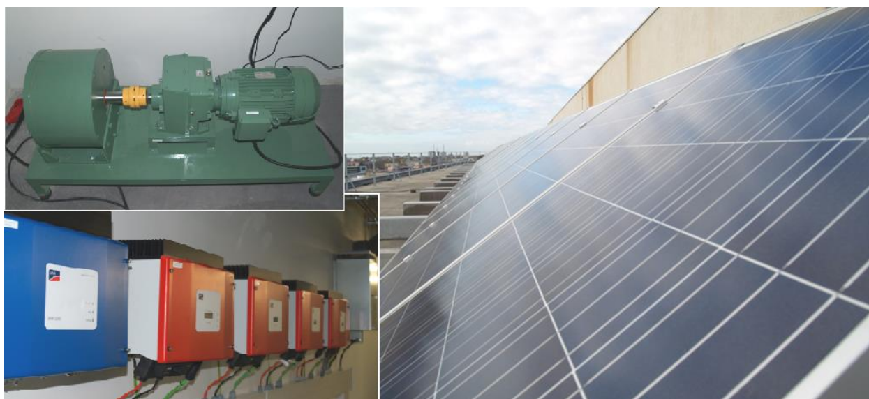
Figure 6. Emulator of the wind turbine (top left corner), solar panels (right) and SMA Sunny Boy inverters (bottom)
