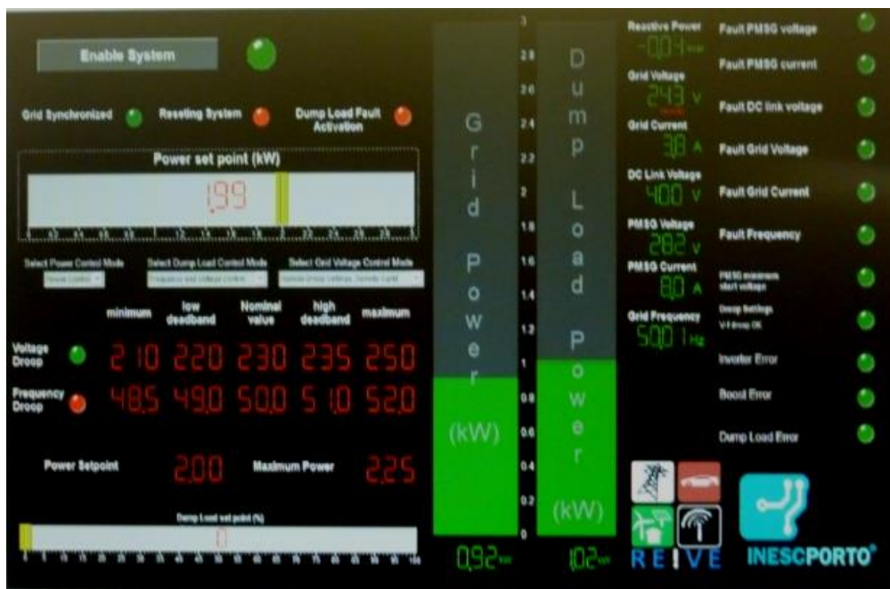
Figure 29: Graphical representation of the micro wind turbine controller – Power injected into the grid and power dissipated in the dump-load
