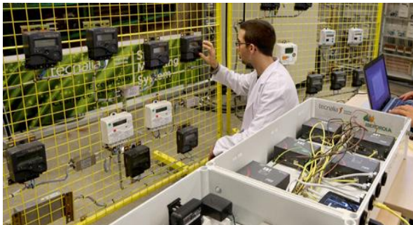
Smart metering communication platform at TECNALIA
