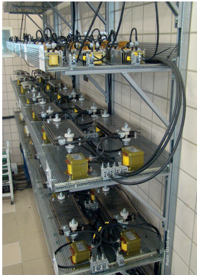
Above: Scaled-down distribution system based on the CIGRE TF C06.04.02 (part of the network branches)
