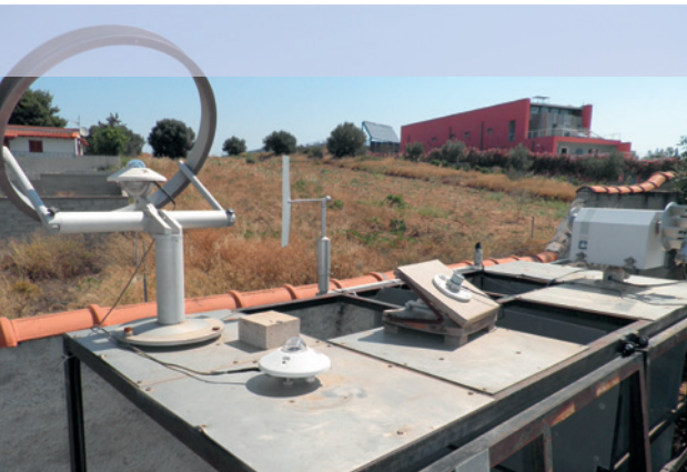
Measuring the meteorological PV testing conditions on the roof of the CRES laboratory
