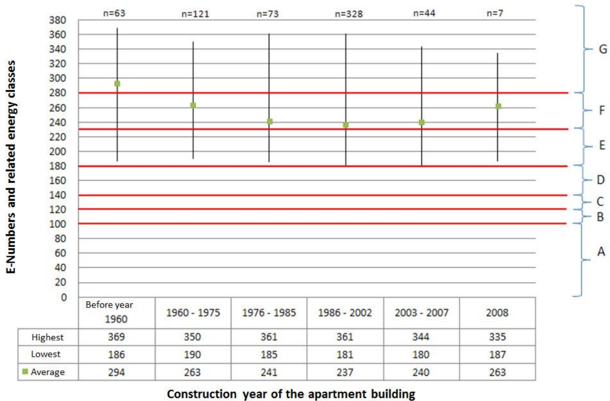
Figure 23: Statistical data of apartment building (located in different part of Finland) related energy consumption and related E-numbers [1]
