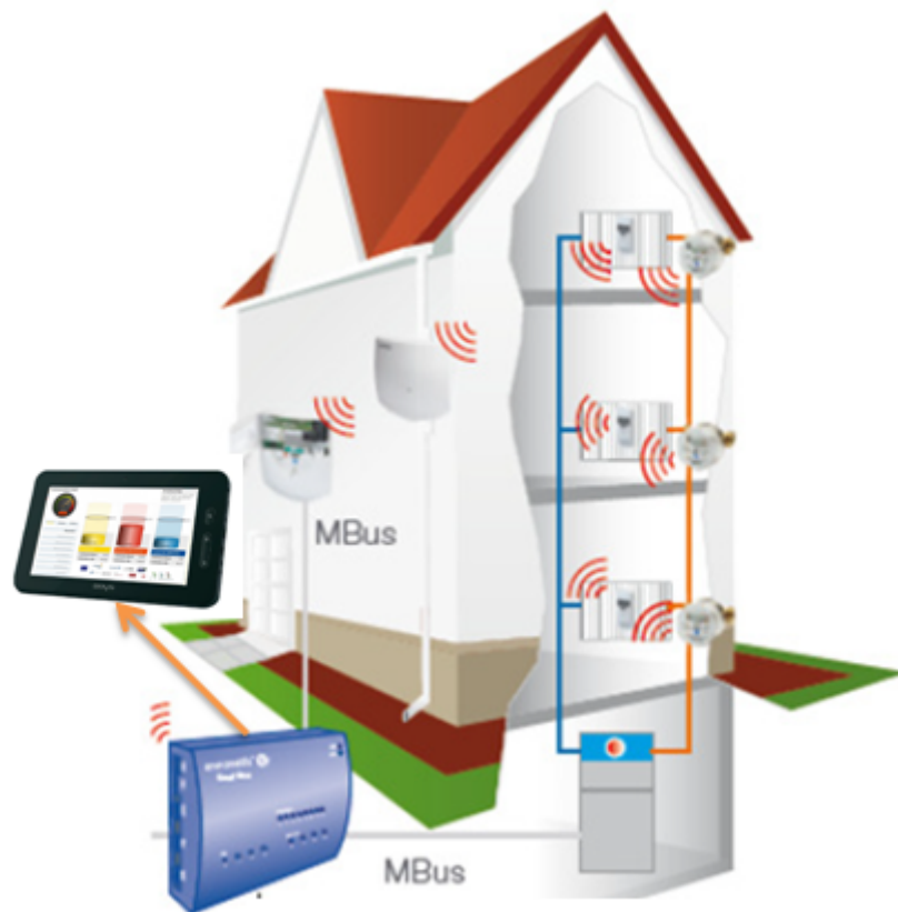
Figure 8. General functionality scheme of option 2 – Data logging and visualisation with Smartbox
