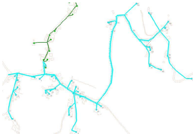
Figure 48: Exemplary depiction of a typical rural LV network. This specific grid can be found in Portugal [35]
