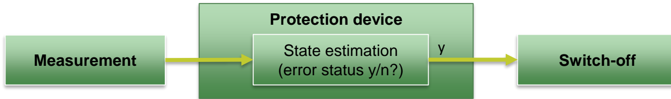
Figure 1: Schematic structure of a protective function with sub-functions
