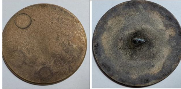
Figure 6: Bronze electrode: Discolorations and deposits on the front and back sides
