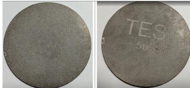
Figure 8: Platinized titanium electrode: Front and back side: spot formation. Source: [3]
