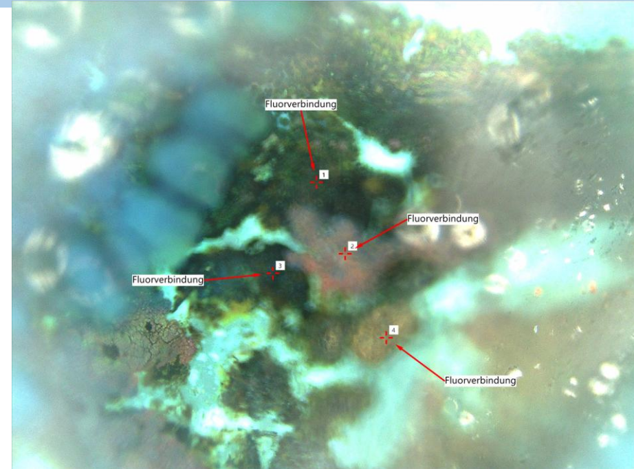
Figure 10: LIBS measurements on the membrane – deposits of copper oxides, chlorides, and hydroxides on the membrane
